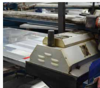
UV Mercury Curing
